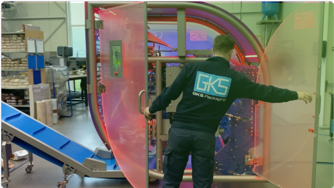
| The LEAF packaging machine lights up in red when it needs maintenance.
